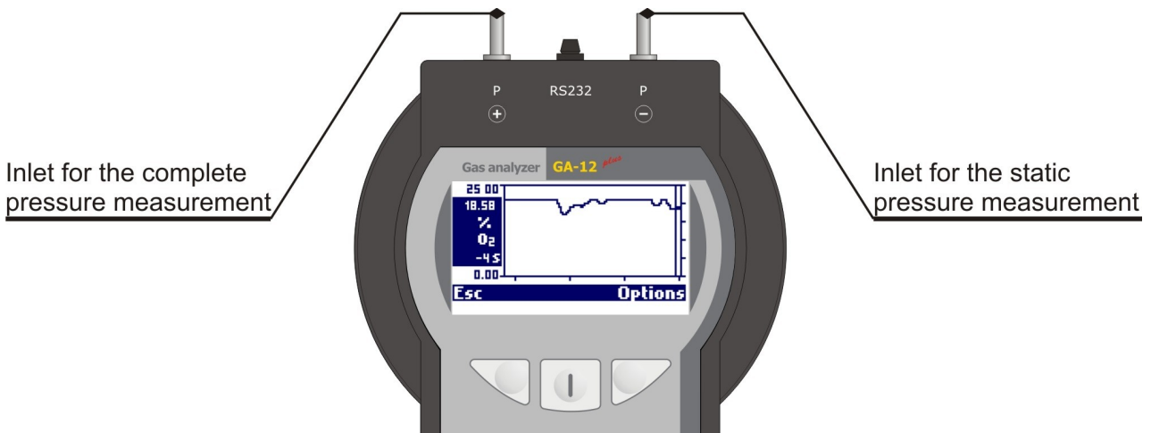
Picture 7. The pressure measurement inlets shown on the GA12-Plus device.
